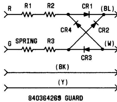
Fig. 2—Current Polarity Guard Schematics
