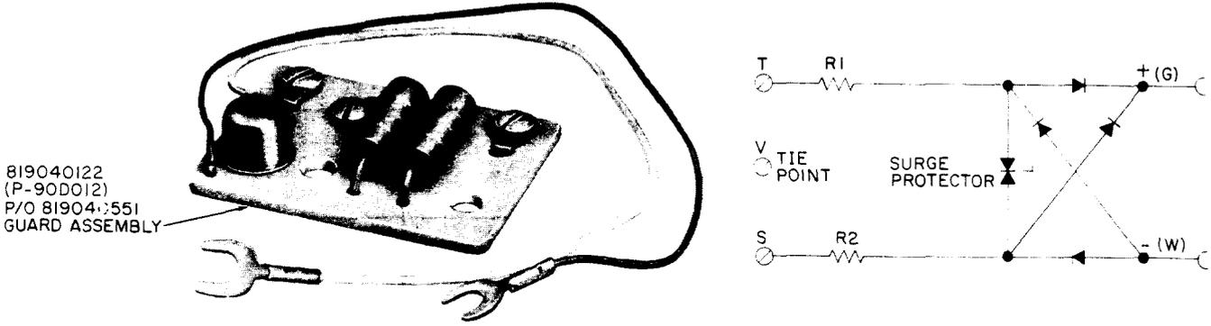
Fig. 5—P-90D012 (MD) Guard Assembly and Schematic
