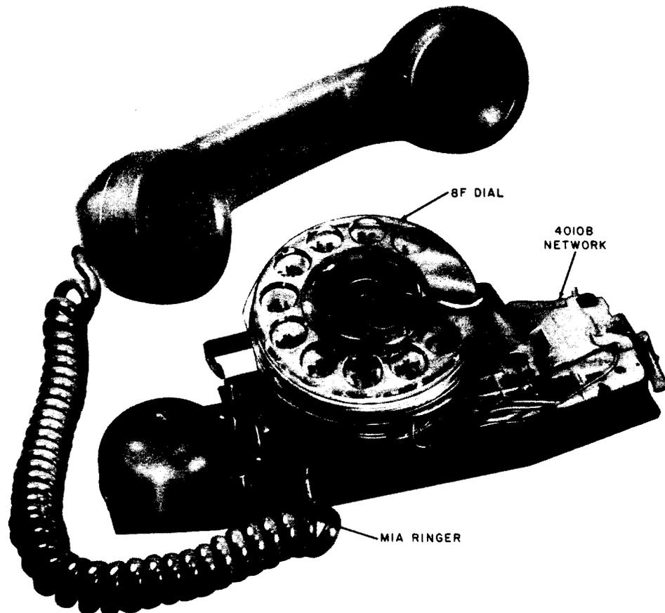
**Fig. 2 — 11C Apparatus Unit**
