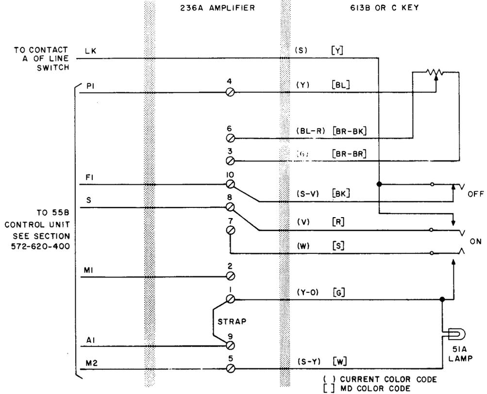
Fig. 17--Typical Connections For 236A Amplifier and 613B or C Key When Used With 611A Key
