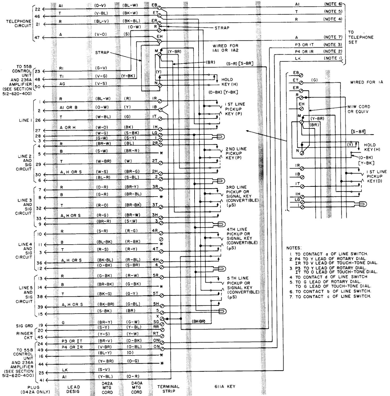
Fig. 18—Typical Connections For 611A Key When Used With 236A Amplifier and 613B or C Key
