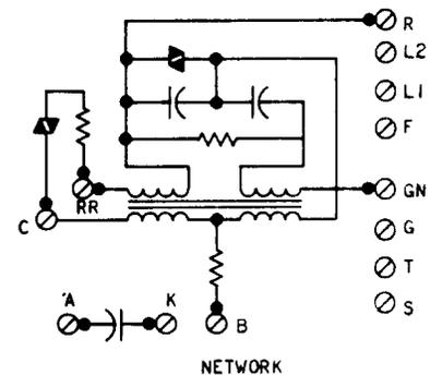
Fig. 1—2660A1M Telephone Set, Connections†
