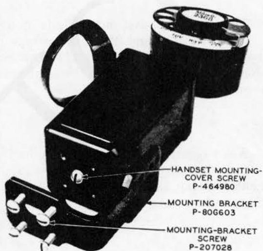
Fig. 17 — Assembly of G-type Handset Mounting and Bracket
