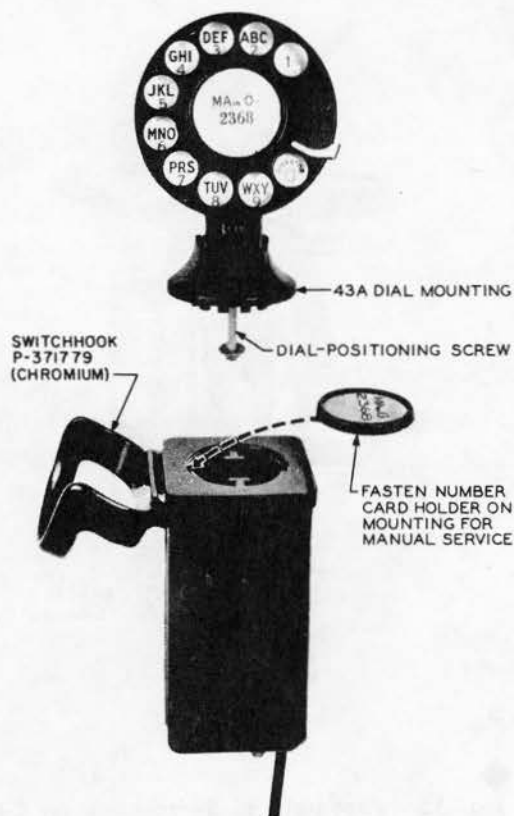
Fig. 16 — Assembly of 43A Dial Mounting on G-type Handset Mounting
