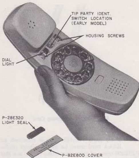
Fig. 10—220A Hand Telephone Set Cover and Light Seal Removed
