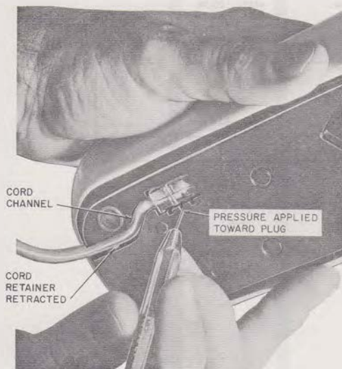
Fig. 16—Removing Mounting Cord From AD1 Telephone Base
