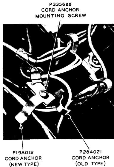
Fig. 4 – Cord Anchors, New Type Cord
