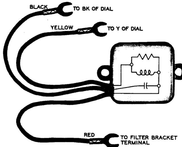
Note: Remove brown-yellow lead from Y of the dial and terminate it on the filter bracket terminal.
