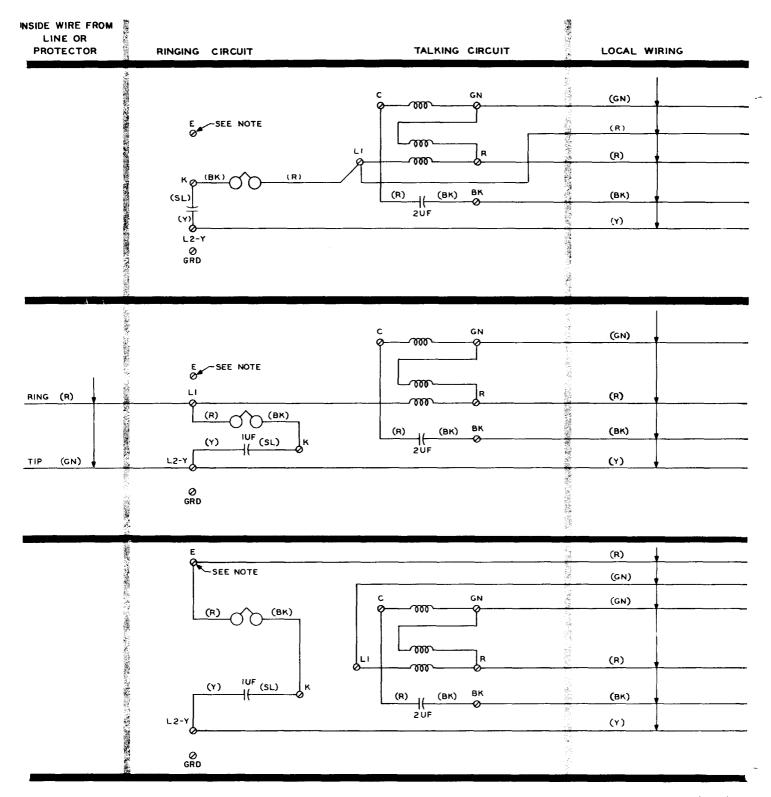
Note: When an E terminal is not normally provided in subscriber sets, use D-161488 connector to connect local wiring to R ringer lead.
