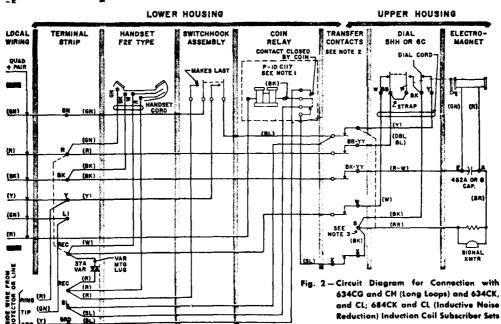
Note 1: The 174CT, GT coin collectors are equipped with P-10E786 coin relays wired as shown above.
