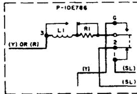
**Note 1:** 176CT, GT coin collectors are equipped with P-10E786 coin relays wired as shown above.
