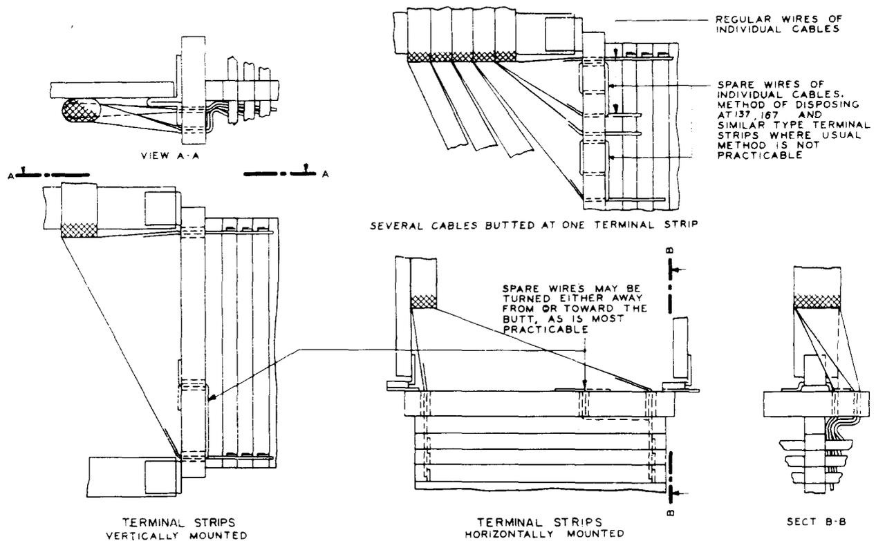
Fig 2—Fanned Form for a Single Terminal Strip
