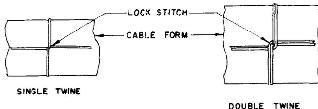
**Fig 25—Starting Stitches for Cable Forms Sewing in Both Directions**
