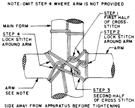
Fig 27B—Cross-Stitch and Lock Stitch Combination for Providing Additional Rigidity at Break-Out of Large Diameter Cable Arms
