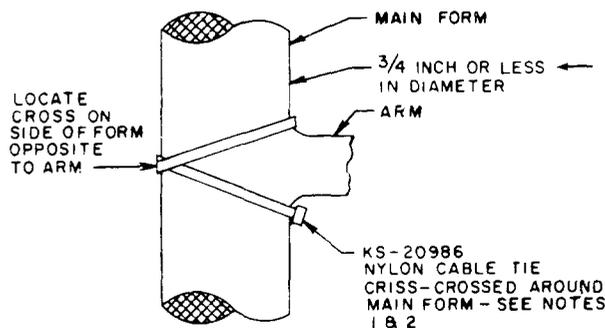
Fig 32—Banding Cable Arm Break-Outs Using Nylon Cable Ties
