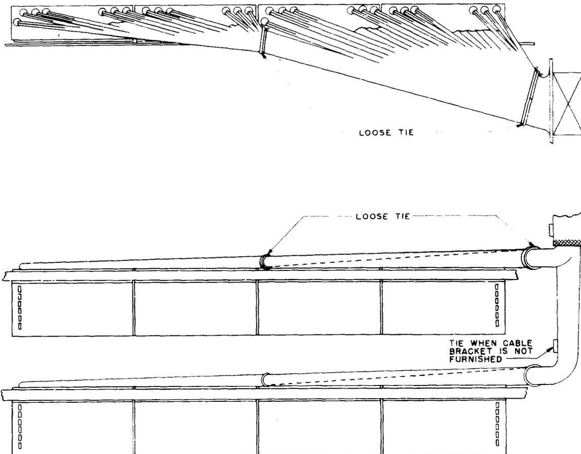
Fig 5—Fanned Forms for More Than One BB6A- and Similar-Type Terminal Strip
