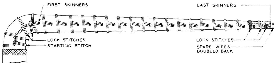
Fig 18—Single-Arm Cable Forms at Right Angles to Butt Sewed With Winding Stitch
