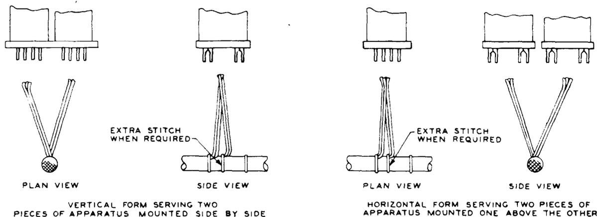
Fig 1—Single Form Serving Two Units of Apparatus
