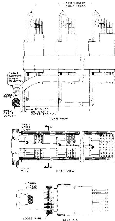
**Fig 6—Terminal Strips—D Type—Loose Wiring and Switchboard Cable Leads**
