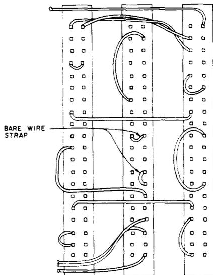
**Fig. 8B—Surface Wire Dress for Connectors Having Vertically and Horizontally Aligned Terminal Arrangements such as the 924-, 925-, 926-, 947-, and Similar-Type Connectors (925-Type Connector Shown)**
