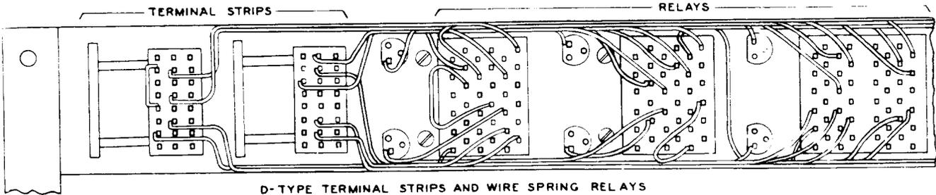
D-TYPE TERMINAL STRIPS AND WIRE SPRING RELAYS
