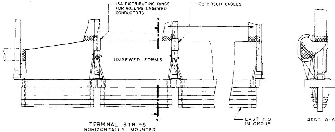
Fig 3—Horizontal Form for More Than One Terminal Strip at Distribution—With Distributing Rings
