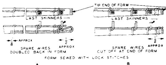
Fig. 10—Spare Wires in Sewed Forms
