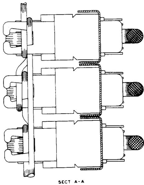
Fig 7—Loose Wiring on Front (Apparatus Side) D-Type Terminal Strips
