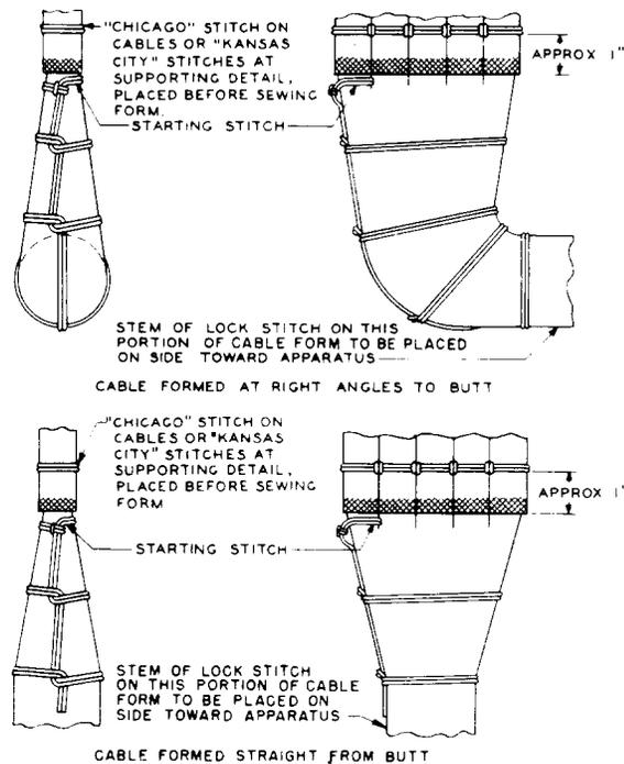
**Fig 12—Two or More Cables Formed Out as a Single Round Arm**
