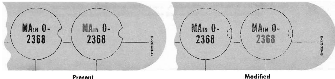
Fig. 1 — Number Card Frames with Number Cards Showing Attachments of Cutouts in Present and Modified Forms (Front)
