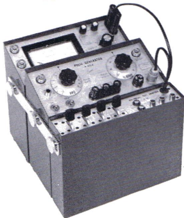
Type P-71 Universal Test Adapter as used with P-672-B Generator and P-652 Analyzer
