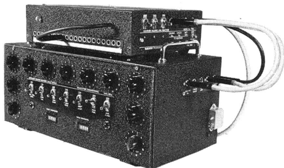
Routiner Multiple Calling Line Selector with Portable Automatic Dialing Routiner and Grade of Service Recorder
