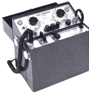
Type P-70 Switch Routing Adapter as used with P-672-B Generator
