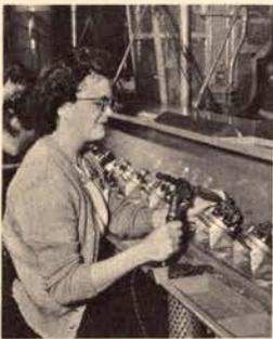
This operator in the network assembly group is shown soldering a resistor to the capacitor on the network assembly. There are 21 Indianapolis employees engaged in similar work.
