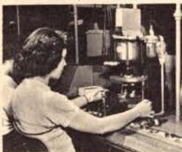
The receiver coil is fastened in place by pressing a coil stop into position. This particular operation is performed at two stations, one on each of the two receiver assembly lines now being operated at Indianapolis.
