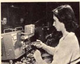
This Indianapolis plant employee is shown adjusting a dial to insure proper pulsing. This adjustment operation is performed at six other stations in the dial assembly group.
