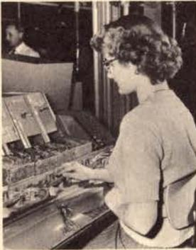
In performing initial stages of operations on switch assembly line, this operator selects switch parts from stock and puts them in the proper order on an assembly fixture. Then other operators add other parts until the pile-up of each switch assembly is complete.
