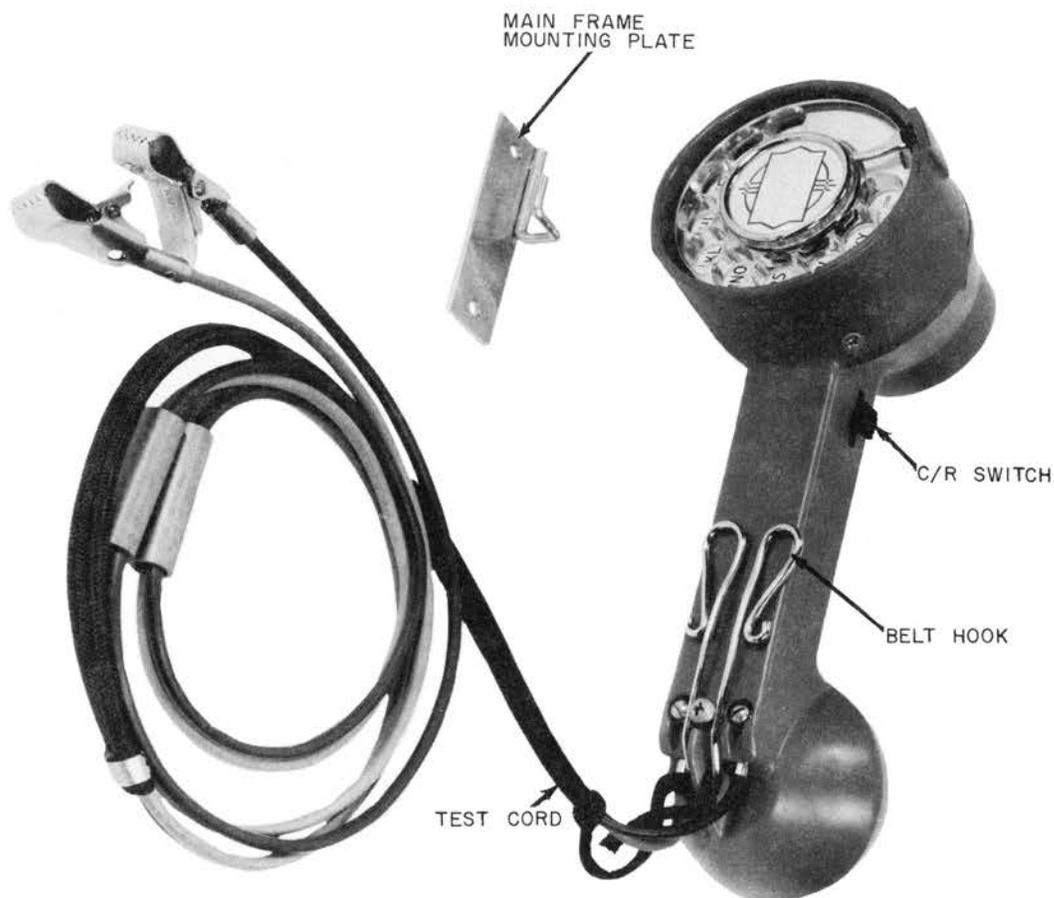
Figure 1. Type 800 Hand Test Telephone.
