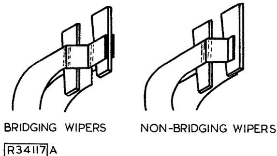
reasonably constant load on the armature as it steps round the bank, and in consequence of this the reduction in armature load at point C in Fig. 3 will be reduced if the wiper assembly includes one or more of the bridging type wipers. Also, in practice the load on the armature will be increased because the bridging type wiper has a larger wiping surface than the non-bridging type, as shown in Fig. 4.
