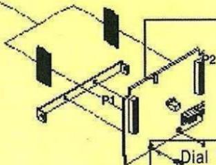
Dial \*#2 before installing or removing option boards.
