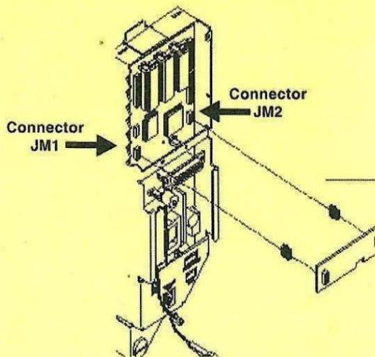
\* Dial \*#2 before installing or removing option boards.
