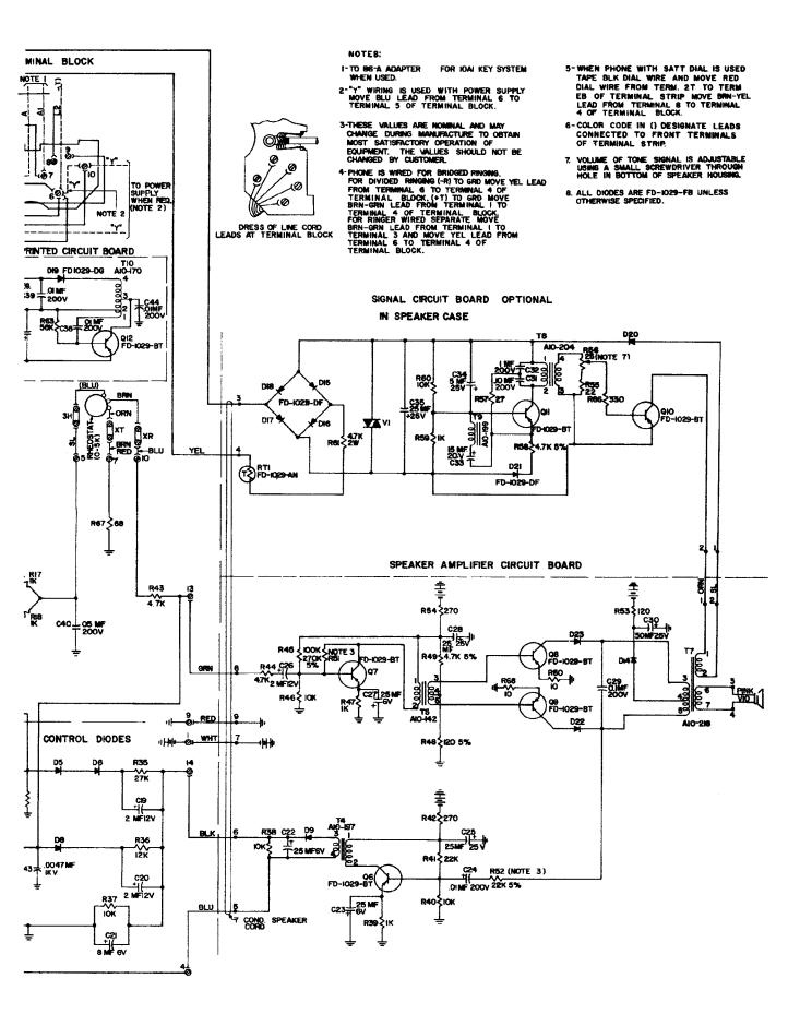
Schematic and wiring diagram of the basic telephone components.
