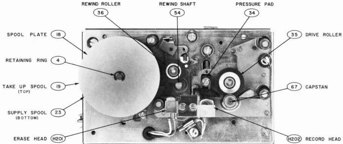
FIGURE 9 TAPE DECK FRONT VIEW, COVER REMOVED
