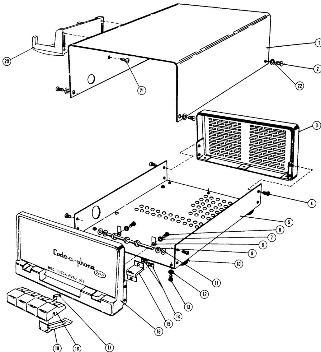
FIGURE 14 CASE EXPLODED VIEW
