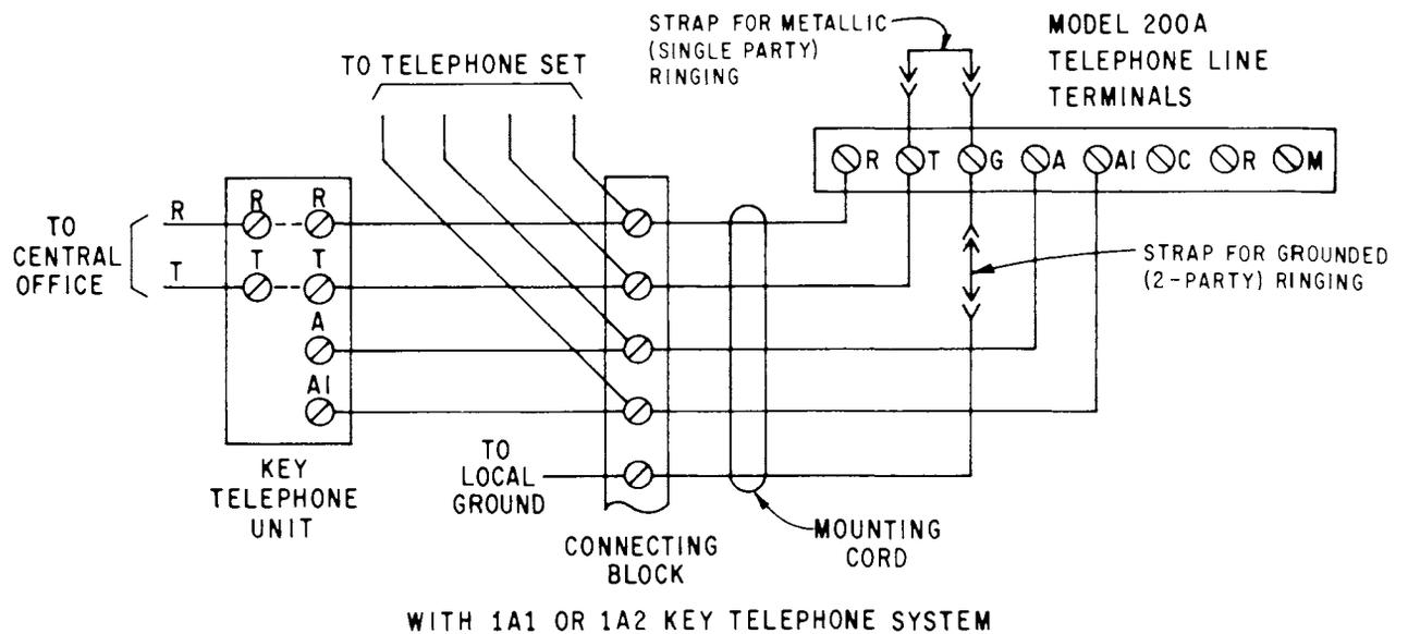
FIGURE 4 CONNECTION INTO KEY TELEPHONE SYSTEMS
