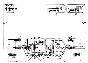
character; that is, they become inert when the receiver is restored to the switchhook at the termination of the conversation. A pilot supervisory lamp  $S^4$ , controlled by relay  $r^2$ , is positive in action, becoming illuminated when the other supervisory signals
