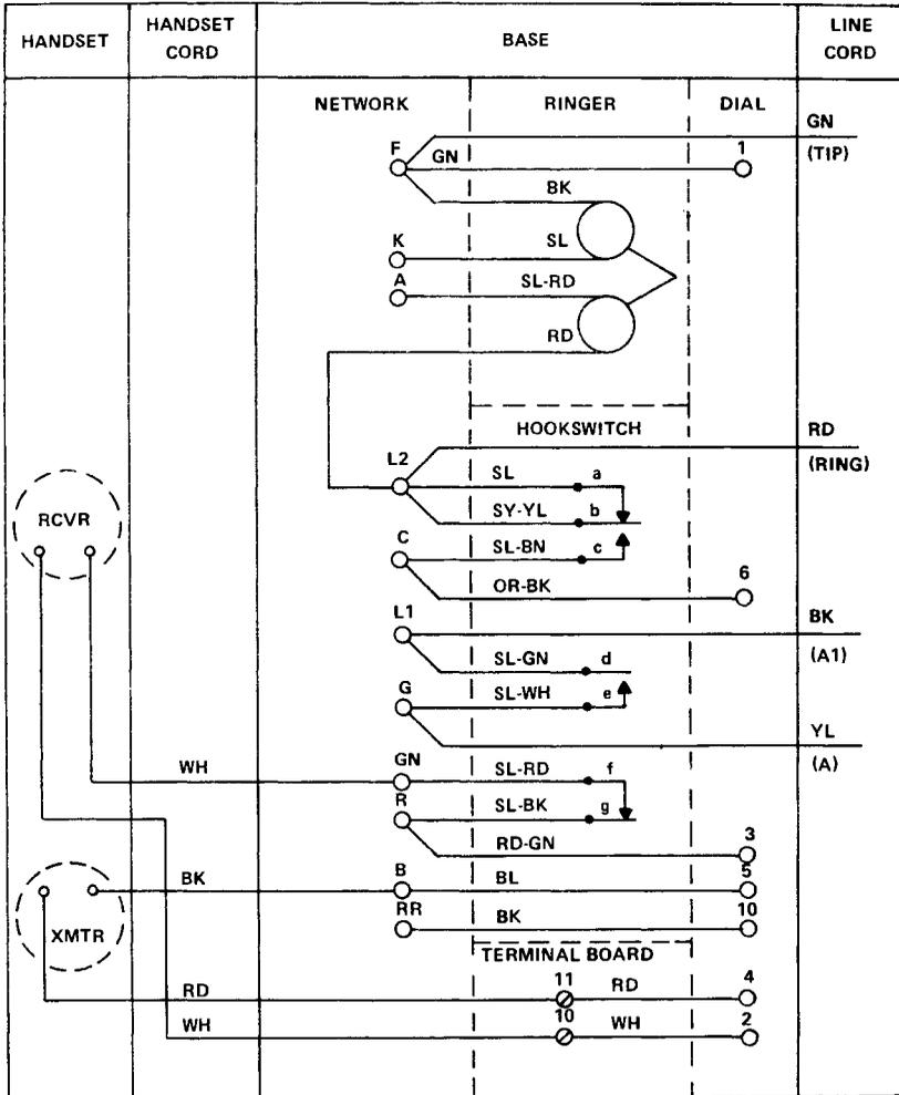
FIGURE 11.05 Circuit Diagram, Model K2500 \*\* ( ) 44
