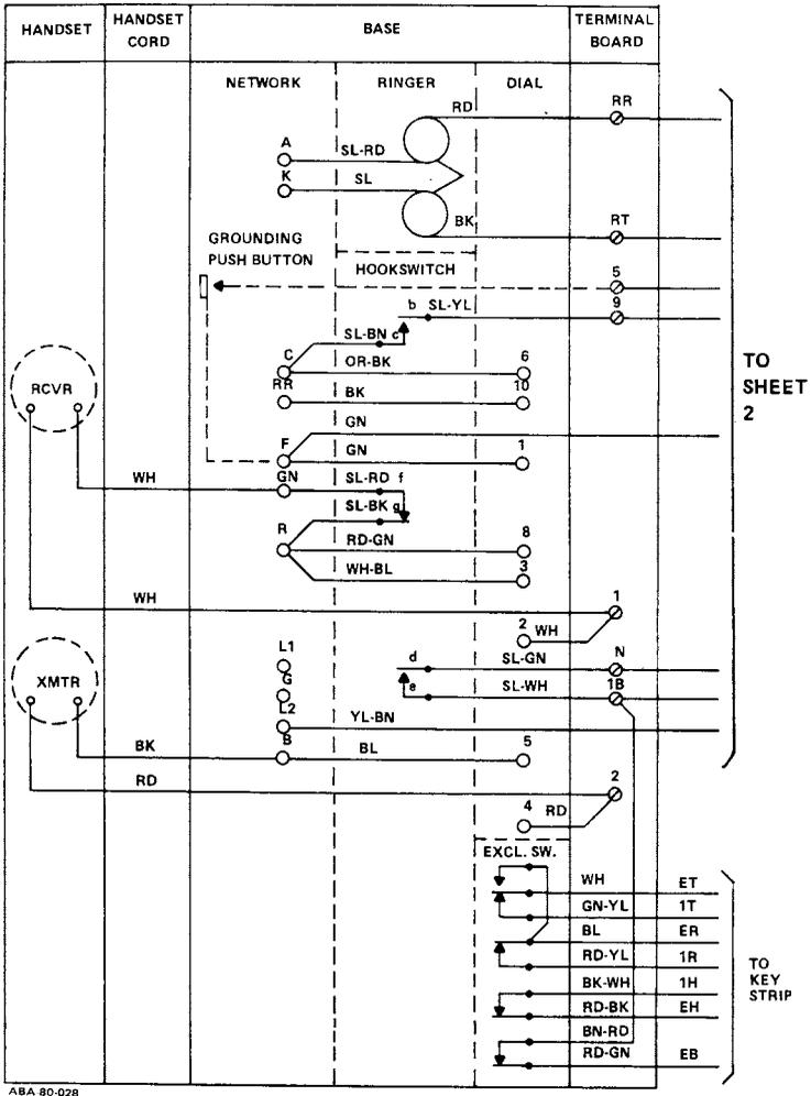
FIGURE 14.02 Circuit Diagram, Model K2565\*\* ( ) 40/41 (Sheet 1)
