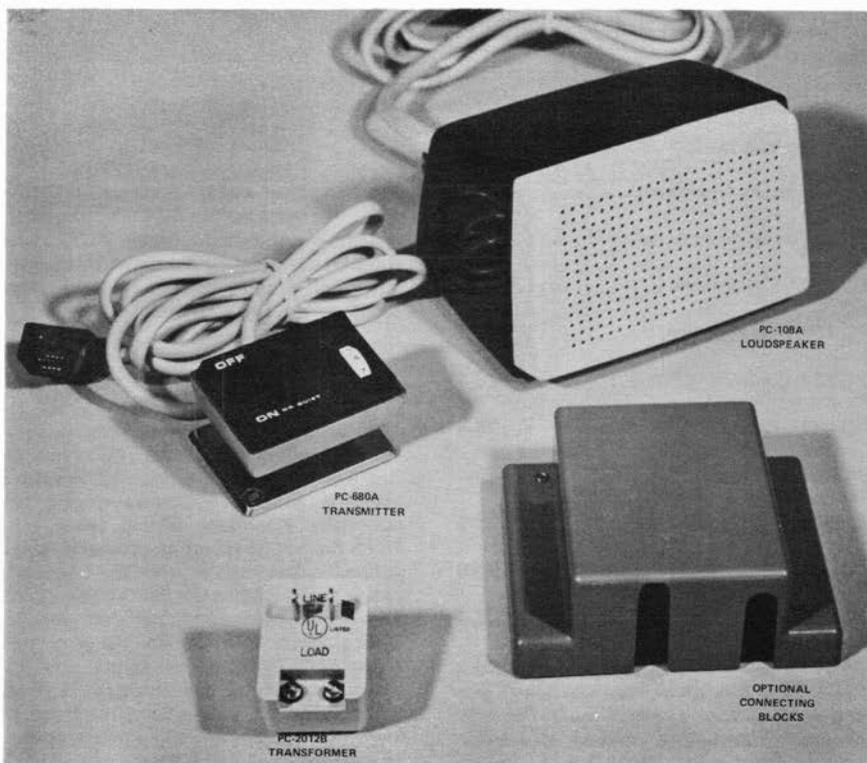
FIGURE 26.00 System - Components of PC-4A Speakerphone
