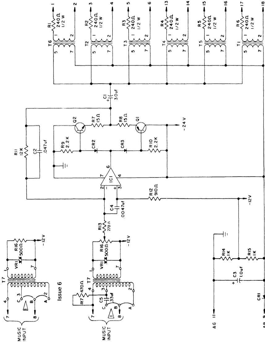
FIGURE 28.15 Circuit Schematic, K-403A KTU
