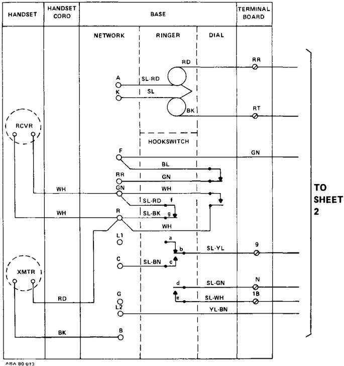
FIGURE 10.01 Circuit Diagram, Model K564 \*\*( ) 30/40 (Sheet 1)
