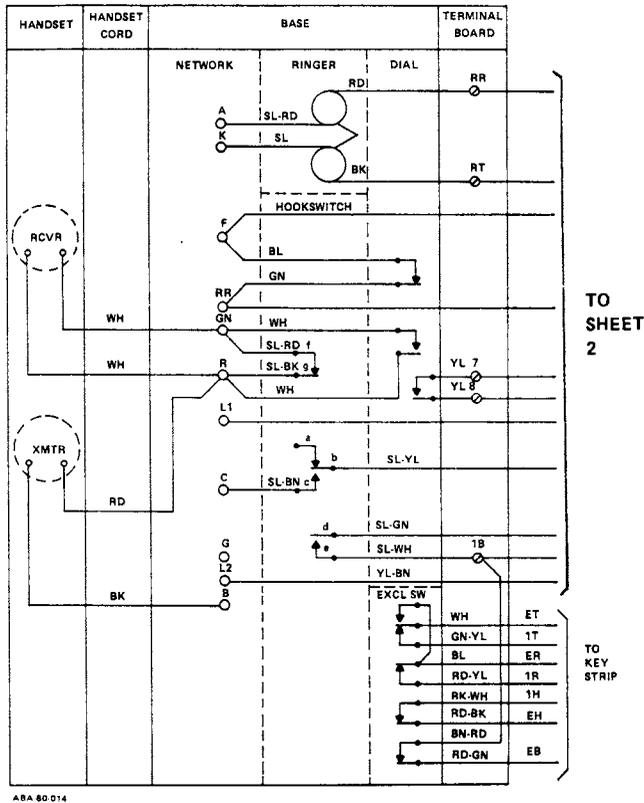
FIGURE 10.02 Circuit Diagram, Model K565 \*\* ( ) 30/40 (Sheet 1)
