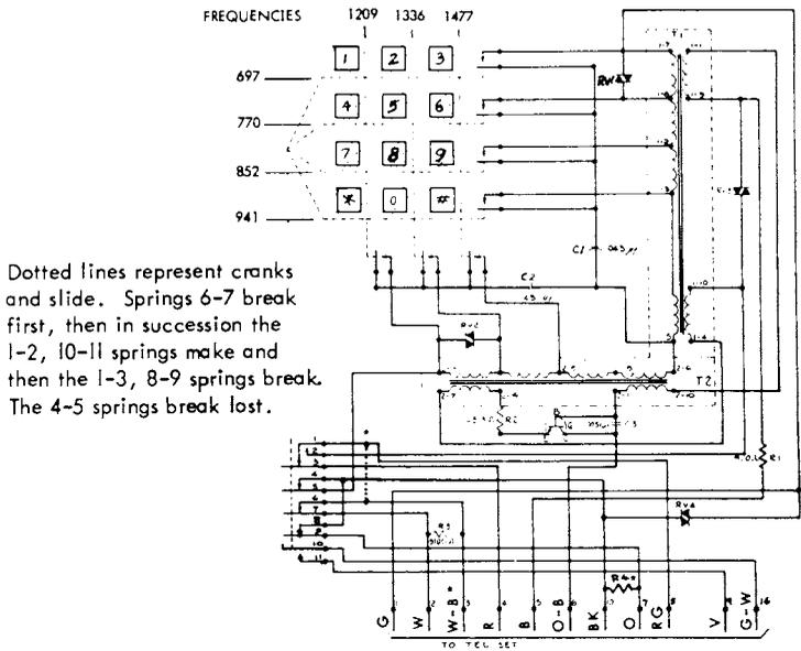
Dotted lines represent cranks and slide. Springs 6-7 break first, then in succession the 1-2, 10-11 springs make and then the 1-3, 8-9 springs break. The 4-5 springs break last.
