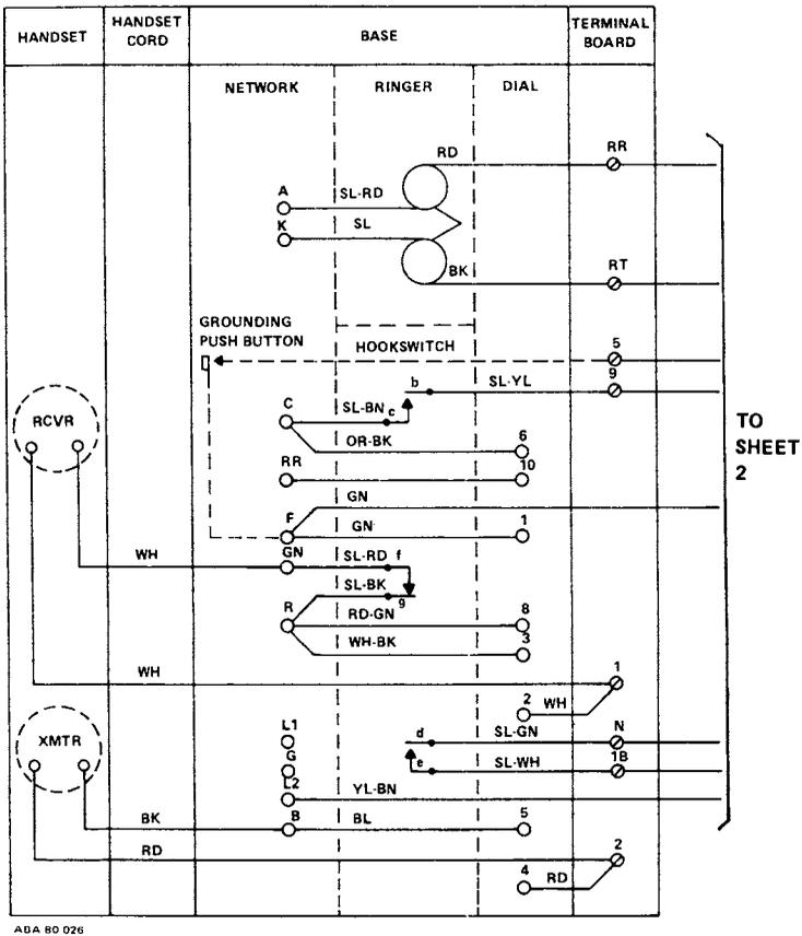
FIGURE 14.00 Circuit Diagram, Model K2564\*\*( ) 40/41 (Sheet 1)
