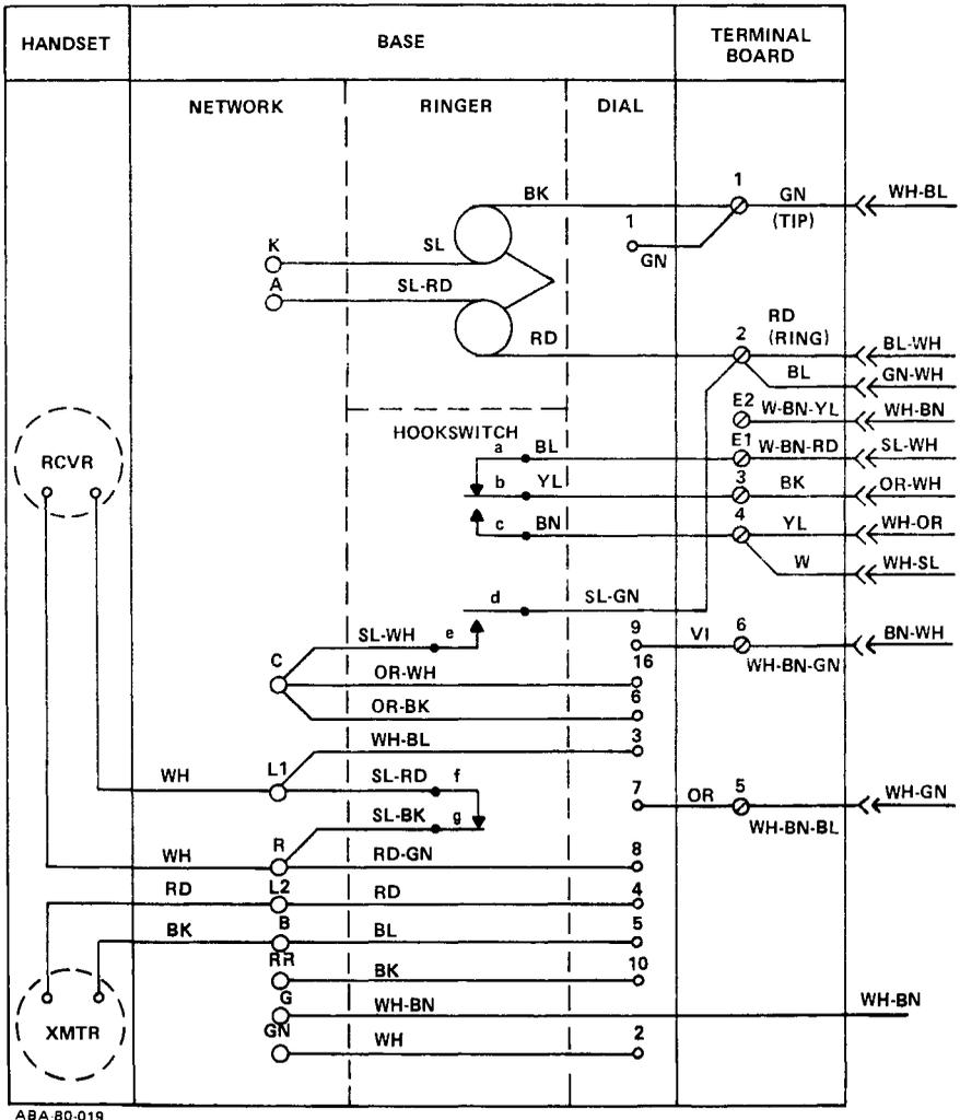
FIGURE 11.04 Circuit Diagram, Model K2500\*\*( ) 39
