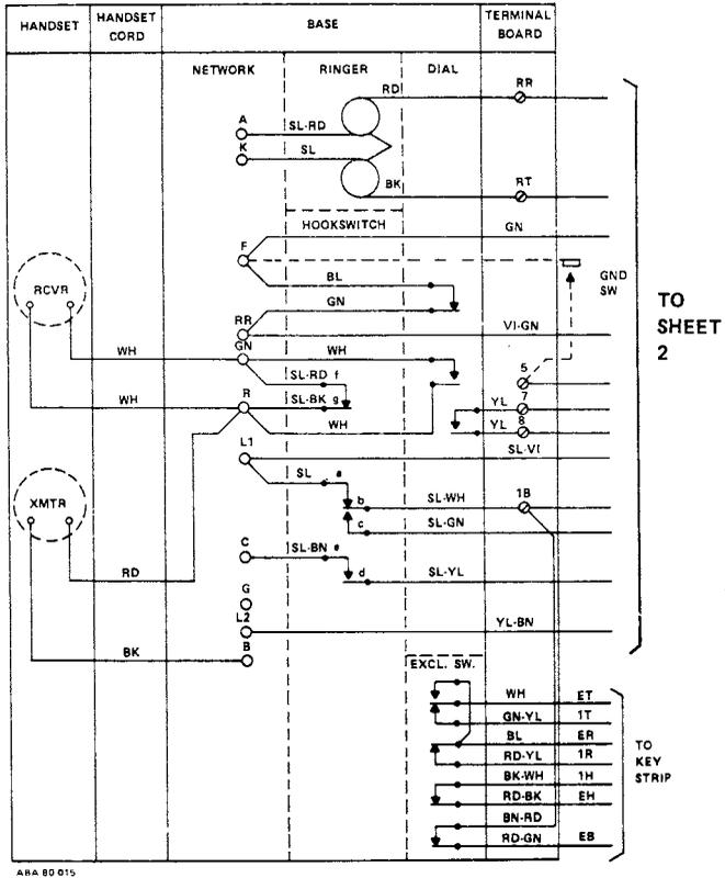
FIGURE 10.03 Circuit Diagram, Model K565 \*\* ( ) 39/42 (Sheet 1)
