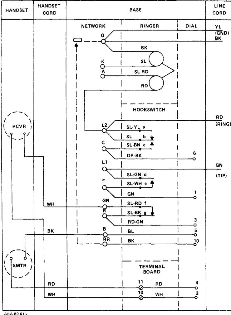
FIGURE 11.01 Circuit Diagram, Models K2500 ( ) 20/24
