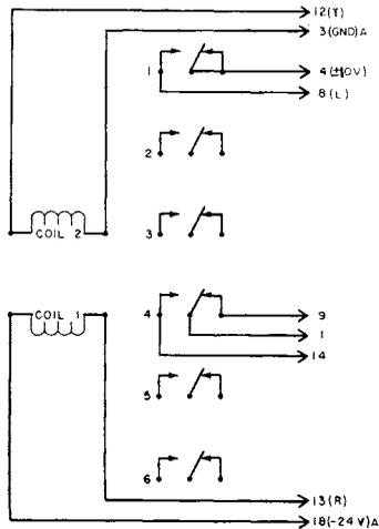
FIGURE 28.14 Circuit Schematic, K-401B KTU
