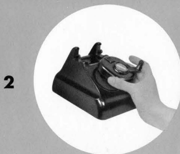
Next it is necessary to change a few wires. No soldering. This changes the circuit to common battery operation. Then remove the generator face plate as shown. Two screws.
