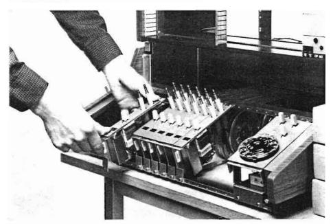
7 Push in the cord-pair units BEH 301 into their positions. Use the middle positions when the maximum number of cordpair units are not to be installed. Screw on the units fastening the lower screws first.
