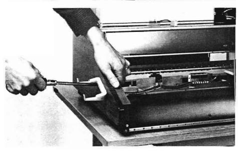
3 Screw the handset holder in place on the left-hand side of the switchboard. Use the following components which are to be found in subset ABZ 151 02.
