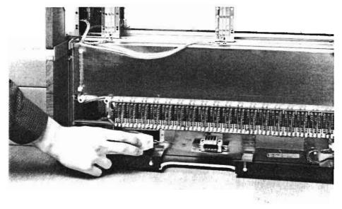
**6** Plug in the plug of the position set into the jack terminal at the rear.
