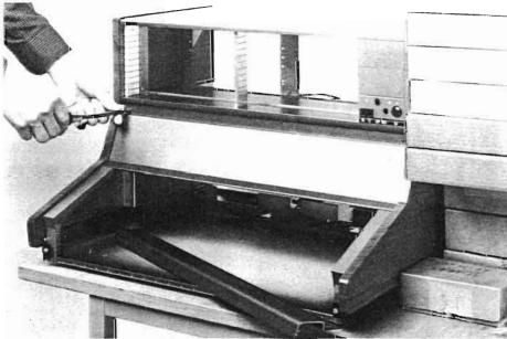
**2** Unscrew the two front plates and the cover plate at the rear.
