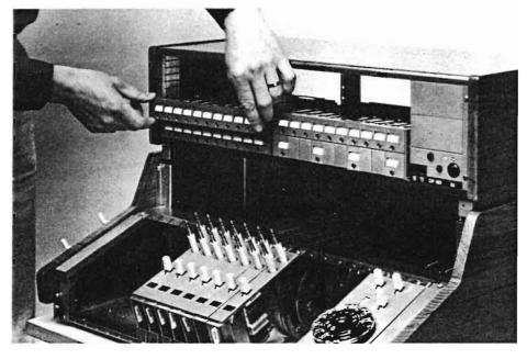
**8** Line units BEF 602 are installed in the line fields beginning at the lowest position.
