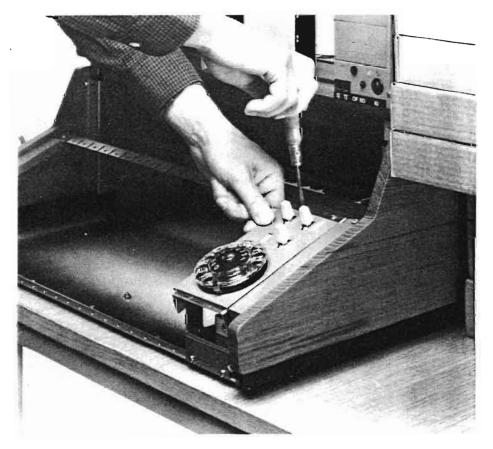
5 Mount position set BEK 251 on the right-hand side. Push the unit's cable with its connection plug through the outlet in the metal wall at the back. Screw the bottom screws in place first, then the top ones.
