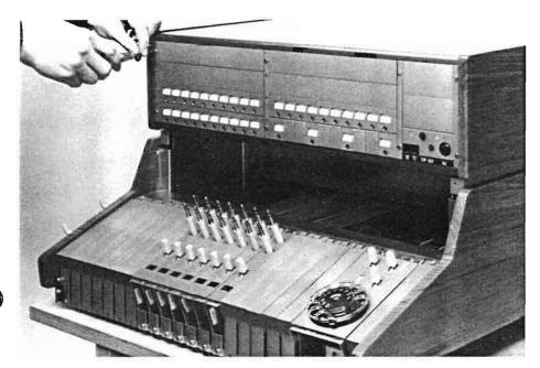
**9** Fit cover strips 957 744/12 in positions where there are no line units. Fasten the fixing plates with 2 screws 05/SBA 139 030/0180 in each.
