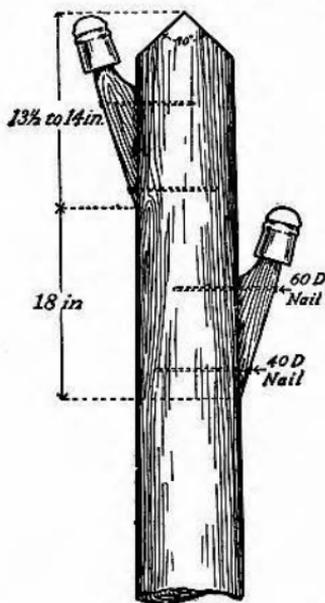
Fig. 5—Location of Brackets on Pole for Straight Lines.
