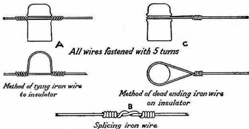
*All joints should be soldered*
