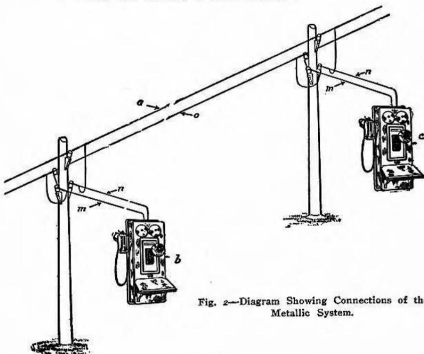
Fig. 2—Diagram Showing Connections of the Metallic System.
