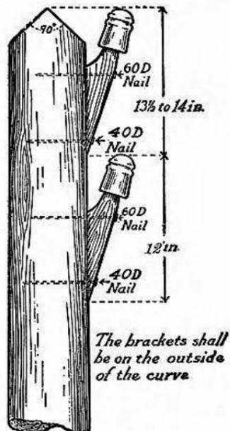
Fig. 6—Location of Brackets on Pole at Curves.
