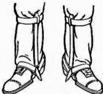
Fig. 28—Method of Attaching Pole Climbers to the Legs.
