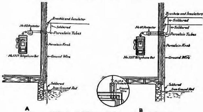
Fig. 43—Methods of Wiring a Telephone Set and Protector: A on a Grounded System; B on a Metallic System.
