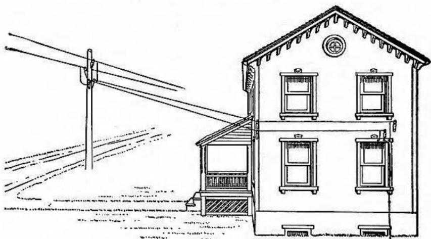
Fig. 42—View Showing How the Drop Wires, When Run Along the Outside of a House, Are Supported on Insulators.
