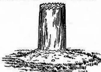
Fig. 18—Earth Should be Slightly Banked Around the Pole as Here Shown.
