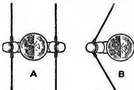
Fig. 30—Method of Fastening the Line Wires to the Insulators—A on Straight Lines; B at Curves.
