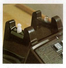
**Models.** There is an optional exclusion feature available on the 6-Button Key Telephone which assures private conversations. Lifting the left-hand cradle plunger 1/4 inch disconnects other telephones from the line.
