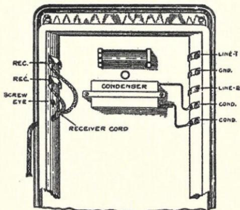
FIG. 7—METHOD OF CONNECTING THE RECEIVER. (THIS FIGURE ALSO SHOWS THE LOCATION AND METHOD OF CONNECTING THE CONDENSER IN THREE BATTERY SETS).
