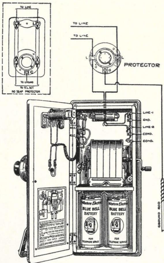
FIG. 10—METHOD OF WIRING SET AND PROTECTOR ON A METALLIC LINE
