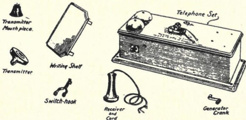
FIG. 1—SET UNPACKED READY FOR ASSEMBLING
