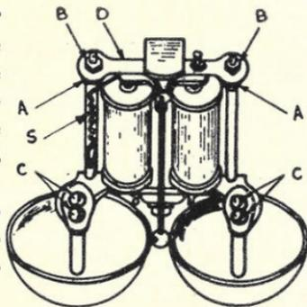
FIG. 14—ADJUSTMENT OF RINGER BY MOVING ARMATURE YOKE
