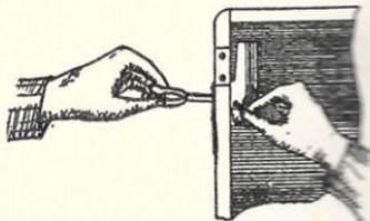
FIG. 6—FASTENING SWITCHHOOK WITH FULCRUM PIN
