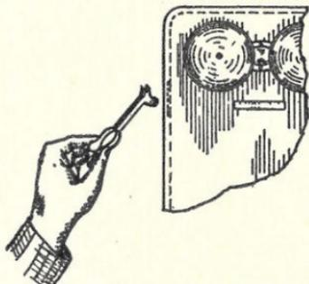
FIG. 5—METHOD OF INSERTING SWITCHHOOK
