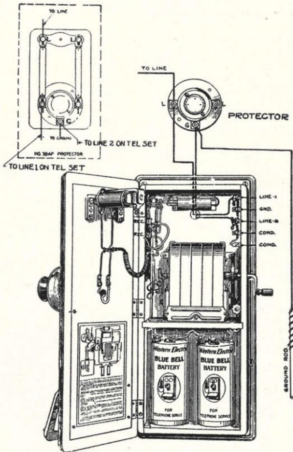
FIG. 11—METHOD OF WIRING SET AND PROTECTOR ON GROUNDED LINE
