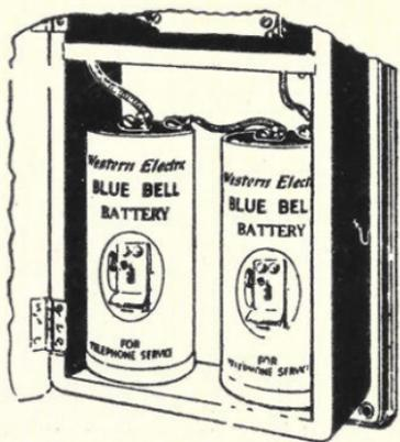
FIG. 12—METHOD OF CONNECTING BATTERIES
