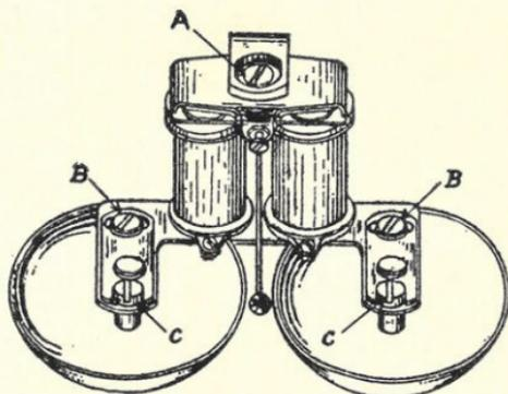
FIG. 13—ADJUSTMENT OF RINGER HAVING SCREW "A"
