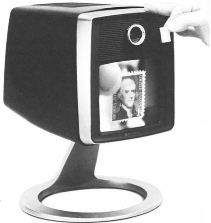
*The simplest add-on for a PICTUREPHONE® set is a single convex lens. Placed over the standard lens, the add-on can be used to provide as much as five times linear magnification of objects.*
