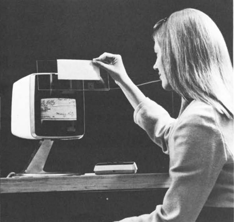
*One of the principal uses of the document magnifier is in banks. A teller can use it to transmit images of checks, for instance, to a person at a central location for verification of signatures.*
