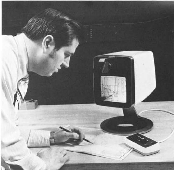
*When the PICTUREPHONE® set is placed on a specially designed rolling base, it can be moved around to view details on a large drawing. A zoom lens allows the user to adjust the magnification.*
