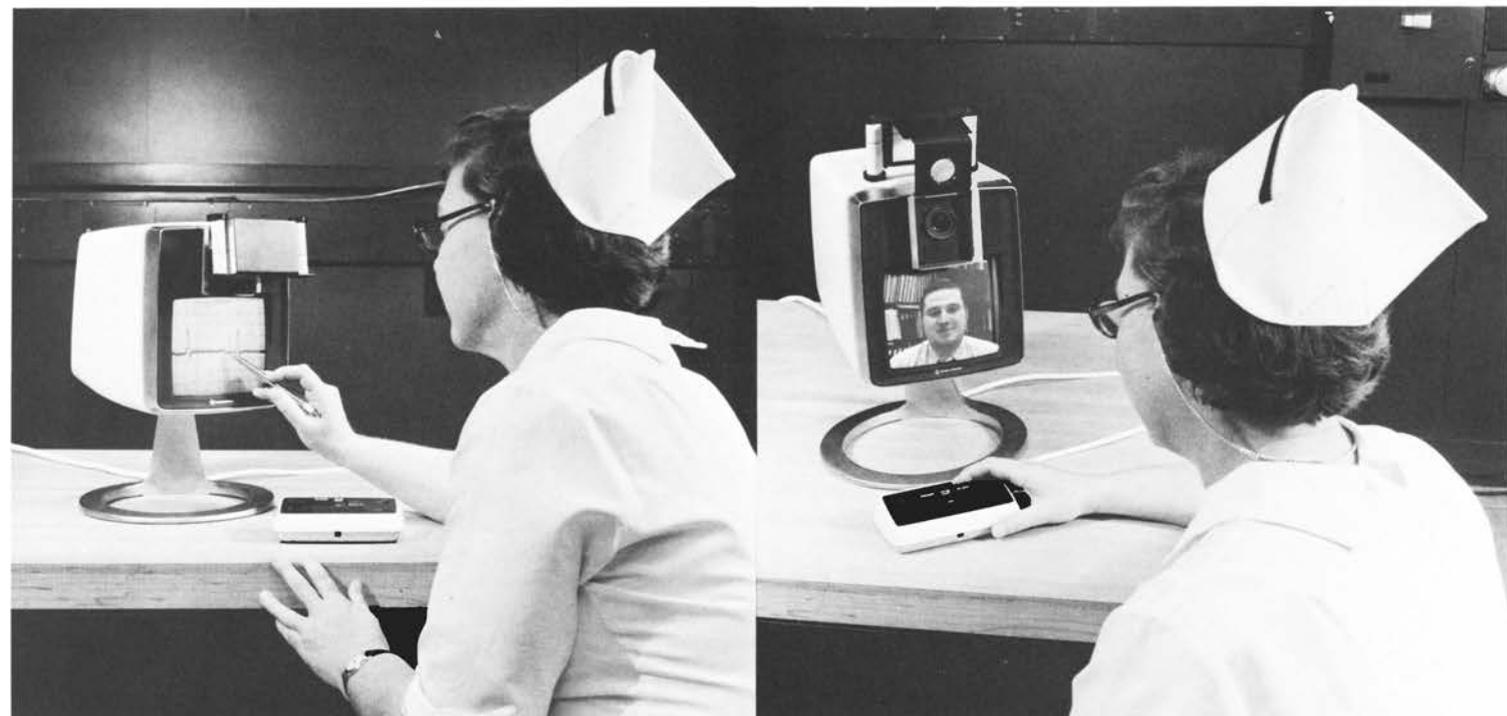
*With the electrocardiogram reader, an EKG record can be transmitted to a medical expert at a remote location (left). The reader consists of a close-up lens and a support that keeps the chart in*
