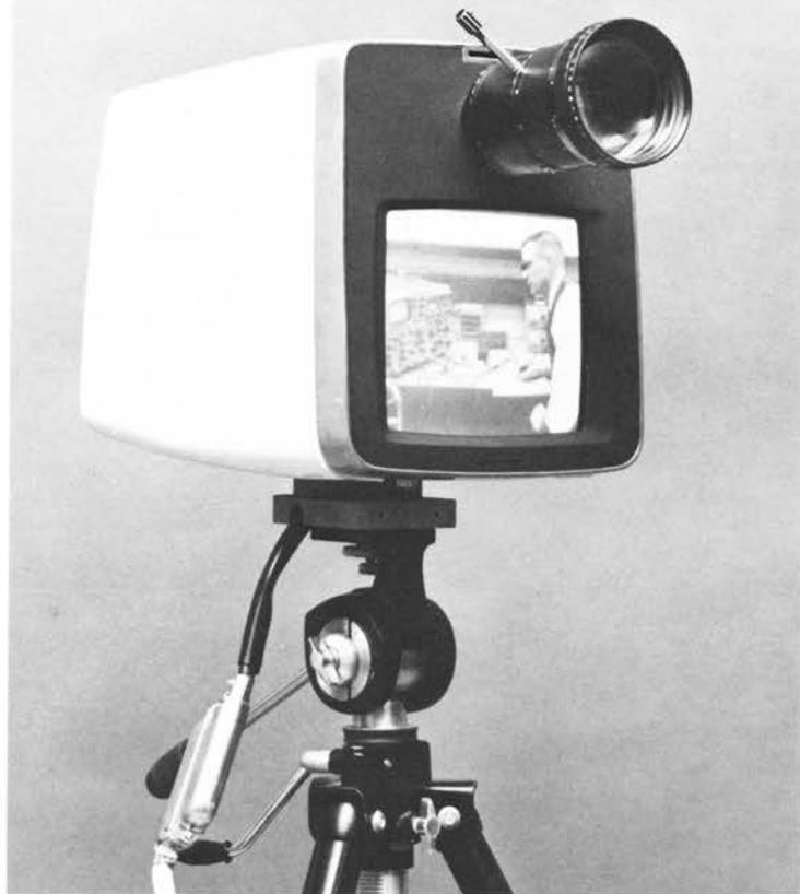
*If the standard base is replaced with a mounting bracket for a camera tripod, the PICTUREPHONE® set can be used in a variety of locations and orientations, much as a studio camera can be.*
