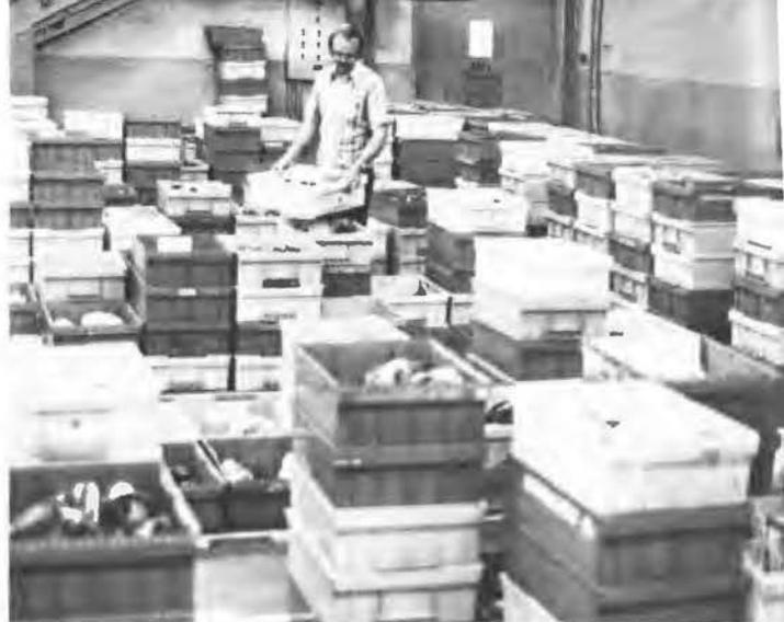
*From telephones to trays. Among the products of recycled ABS made from telephone housings are warehouse trays. At Western Electric's Nashville Service Center, such trays are being used to store and transport more housings for recycling.*
