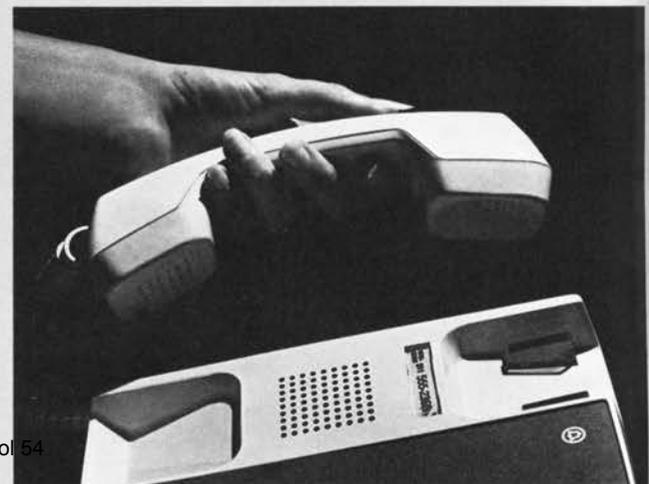
The MAAP in the DIMENSION PBX is used to change telephone features and line pickup assignments and to diagnose system problems.
