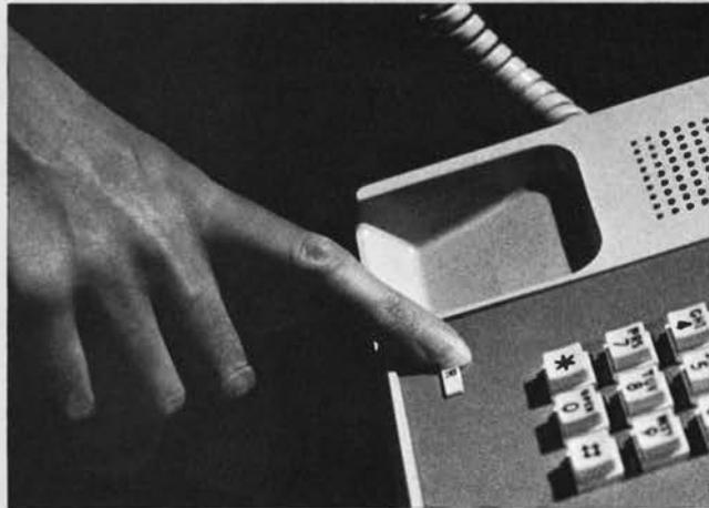
The Recall button eliminates the need to flash the switchhook to access special features.
