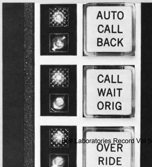
Custom-calling feature buttons replace dial codes. For example, after receiving a busy signal, a DCTS customer has several options: press Automatic Callback and when the line is free be called back automatically; press Call Waiting-Originating to send a special tone that lets the busy extension know a call is waiting; or press Executive Override to talk to the called party immediately.
