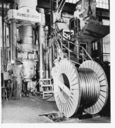
Applying lead sheathing to telephone cable in a Western Electric plant. The finished cable is guided onto the reel in the foreground.
