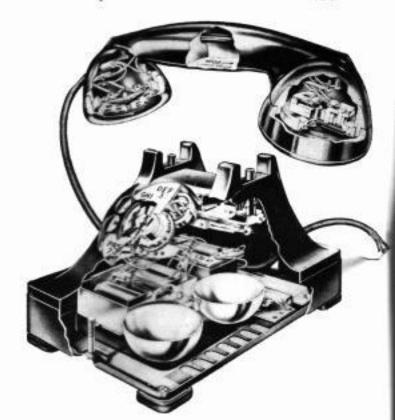
Cut-away view of a modern combined dial telephone set. This type of instrument contains 433 parts, each of which must meet rigid standards of accuracy, precision and endurance.
