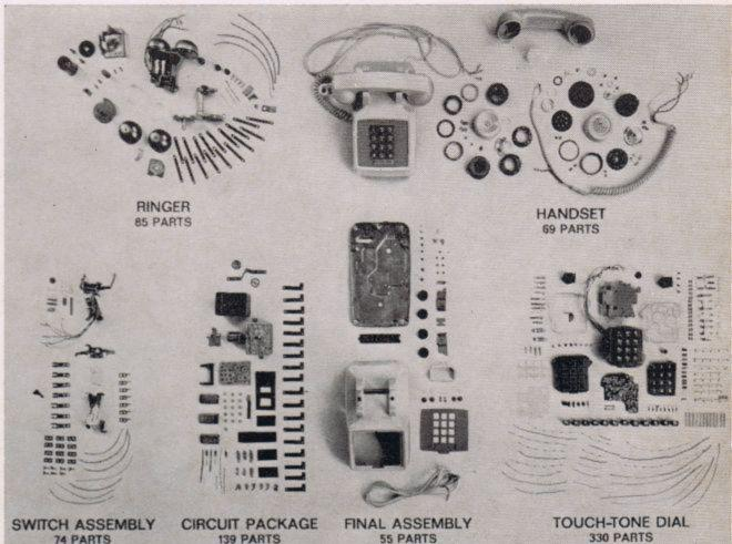
■ The Touch-Tone telephone, manufactured by the Western Electric Co. for the Bell System, is made up of 752 parts. This is a total count of physical parts only. Chemically, there are only 35 elements present, but this is
