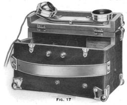
with a hand telephone as illustrated, two cells of dry battery, a buzzer, and a four or five bar hand generator as specified. The case when closed is fastened by two catches. Each set has a carrying strap provided with buckles, so that a shoulder strap can be added if desired.
