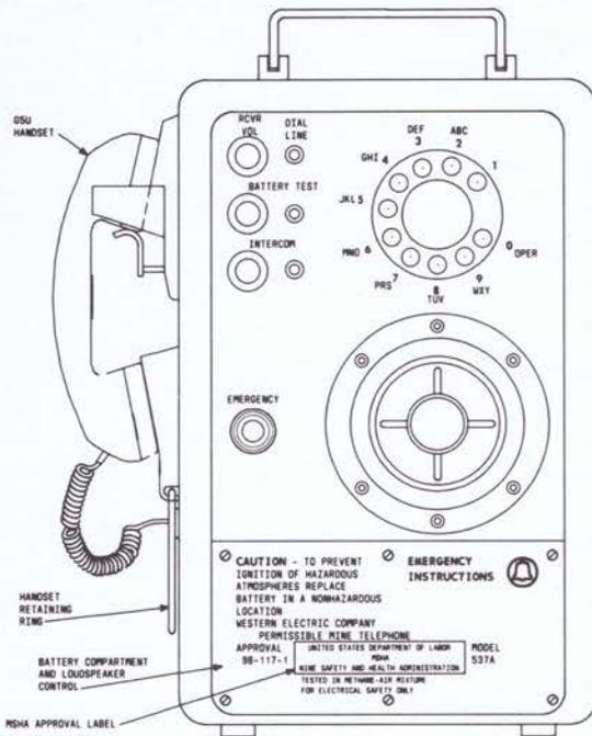
A rotary dial telephone set equipped with a G5U handset, a flush-mounted loudspeaker, a battery test button, a RCVR VOL pushbutton, an emergency button, and is powered by a 12-volt dry cell battery housed in the lower compartment of the telephone set and provides sufficient power for approximately 3 months when handling an average of 29 incoming and 48 outgoing calls per day with an average holding time of 1 minute per call.
