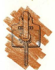
You can temporarily rest the handset in the cradle vertically on the front of the set if you have to leave the phone in the middle of a call.
