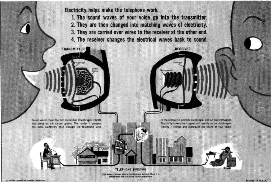
Sound waves make the thin metal disc (diaphragm) vibrate and press on the carbon grains. The harder it presses, the more electricity goes through the telephone wire.
