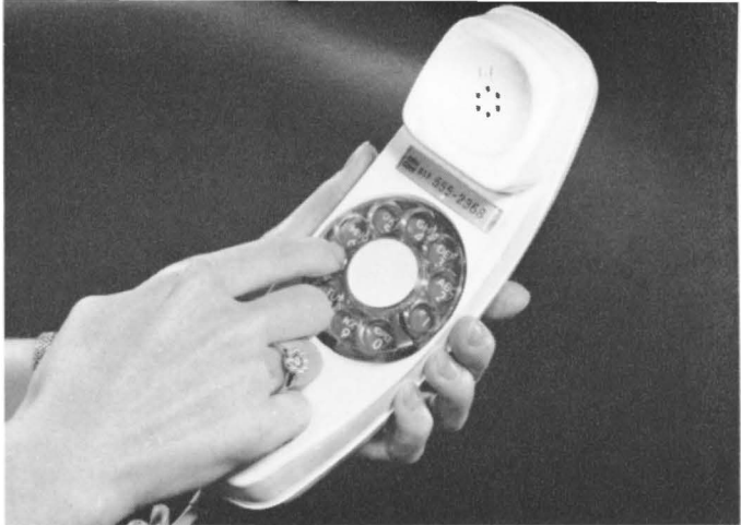
Near dial is a recall button which allows you to make call after call without hanging up.
