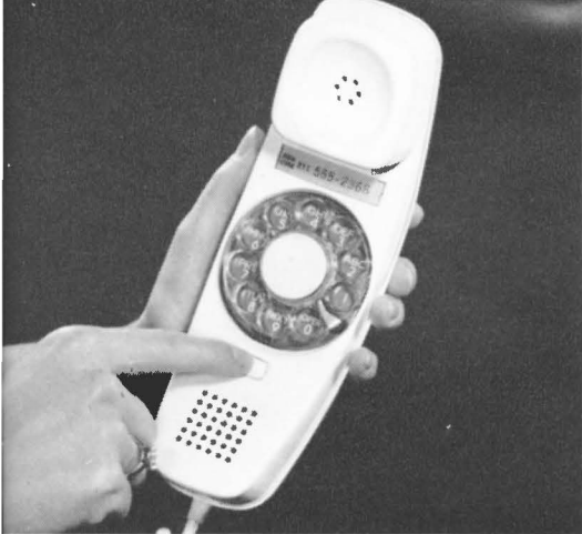
Near dial is a recall button which allows you to make call after call without hanging up.
