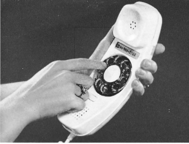
Light-weight Trimline phone has dial in handset, making dialing easier, more convenient.
