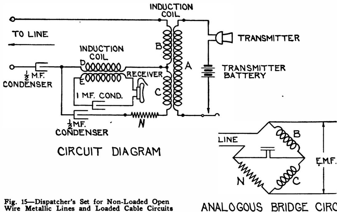
Fig. 15—Dispatcher's Set for Non-Loaded Open Wire Metallic Lines and Loaded Cable Circuits
