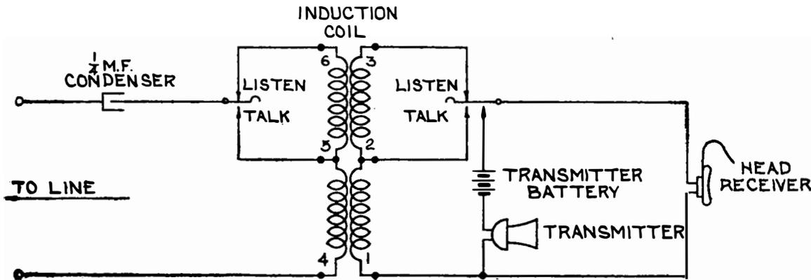
Fig. 12—Circuit Diagram for a Way Station Set for Open Wire Lines
