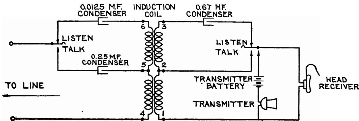
Fig. 13—Wiring Diagram for Way Station Set for Loaded Cable Dispatching Circuit
