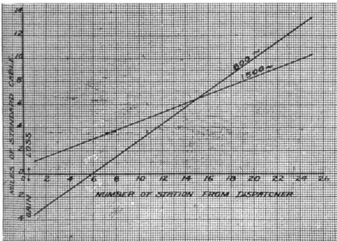
Fig. 10—Circuit Loss Curves for a 100-Mile Line
