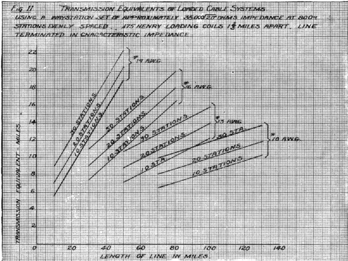
Fig. 11—Transmission Equivalents of a Loaded Cable System
