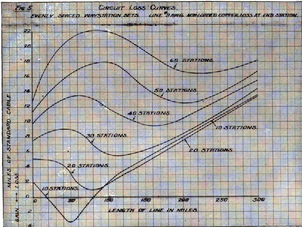
Fig. 5—Circuit Loss Curves, for Last Station on the Line
