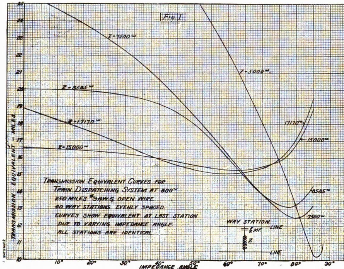
Fig. 1—Transmission Equivalent Curves for Train Dispatching
