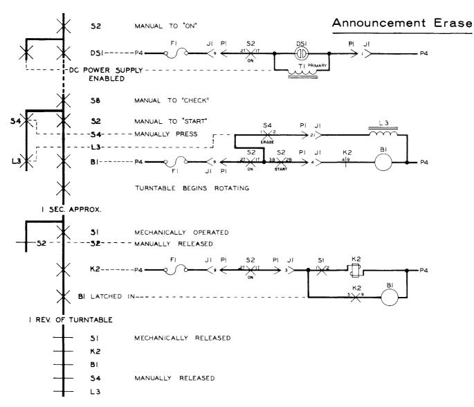
Figure 1. Announcement Erase Functional Diagram.
