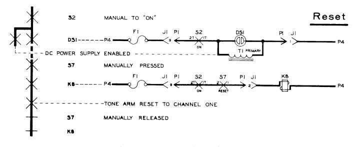
Figure 8. Reset Functional Diagram.
