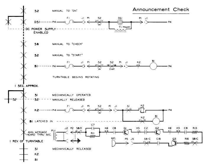
Figure 3. Announcement Check Functional Diagram.
