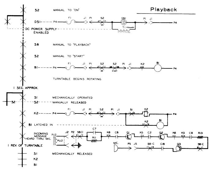
Figure 6. Playback Functional Diagram.
