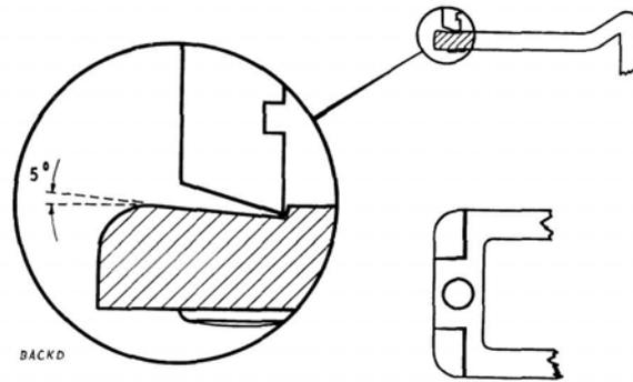
★FIG. 3. ARMATURE WITH 5° TILT
