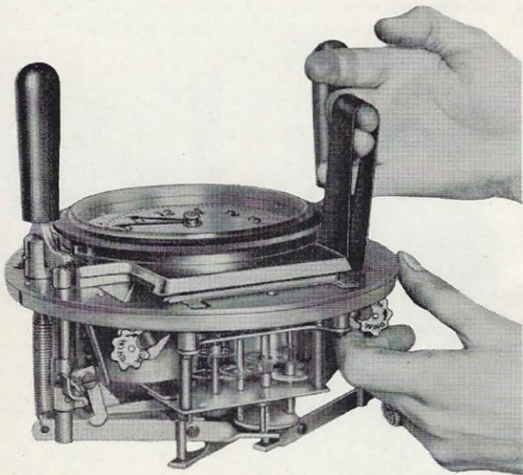
Put instrument back in its case and replace the ticket plate.
