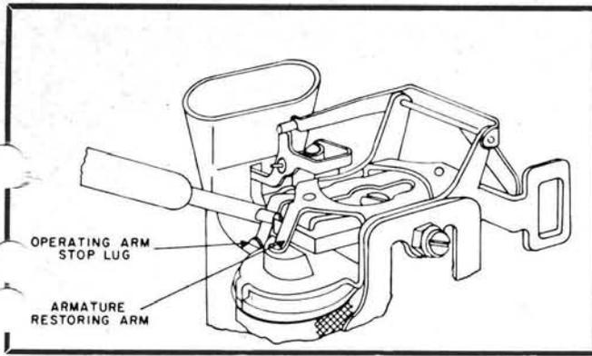
Fig. 7 Adjusting coin relay operating arm stop lug for proper clearance.
