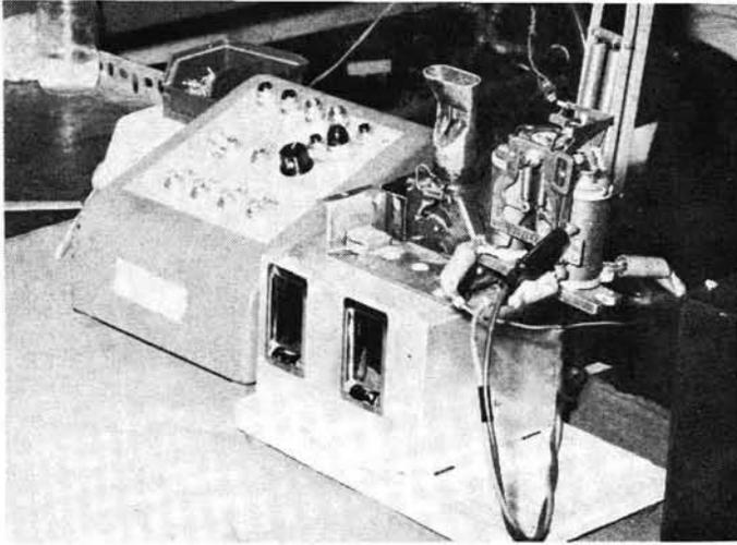
Fig. 9 This test set used in final adjustment of the coin relay was constructed by a telephone repair center.
