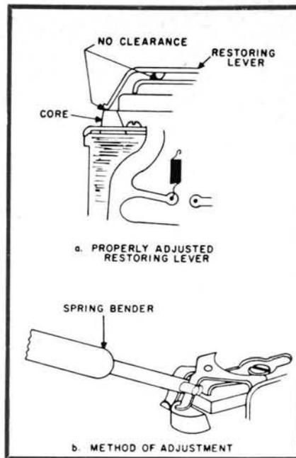
Fig. 6 The clearance adjustment is highly critical.
