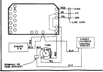
CONNECTIONS FOR A - TIP STATION, FOR A - RING STATION CONNECT TUBE AND RINGER LEADS AS SHOWN BUT CONNECT RING OF LINE TO L-1.
