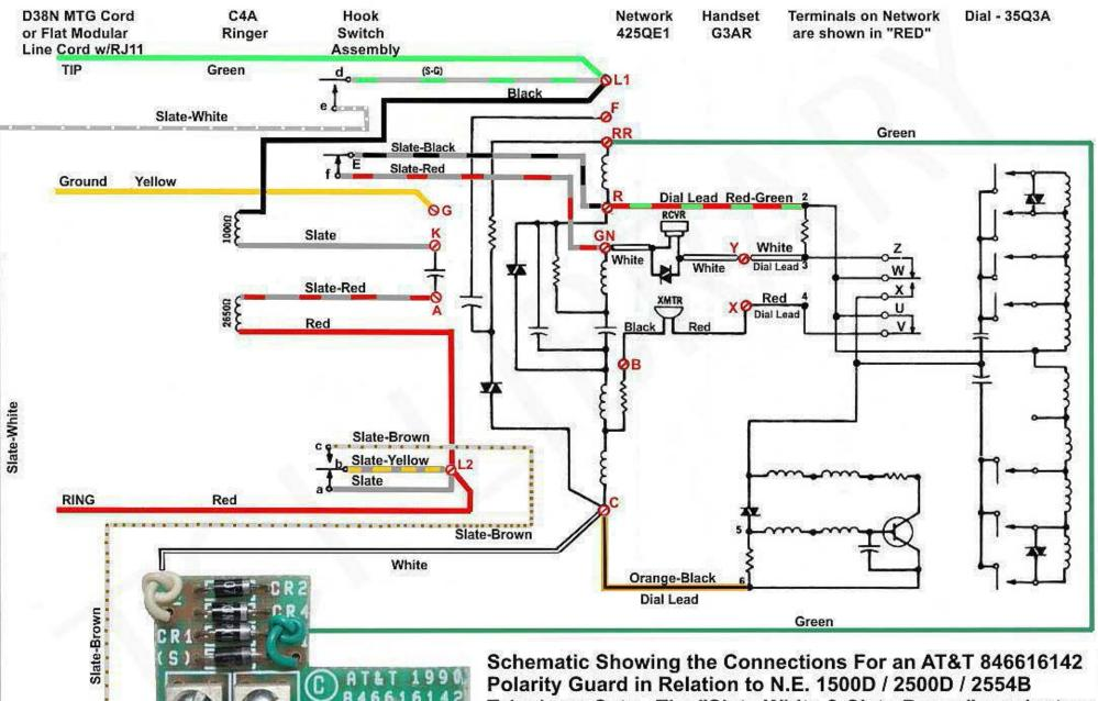
Telephone Sets. The "Slate-White & Slate-Brown" conductors attached to the "Polarity Guard" are leads from the switch hook assembly.
