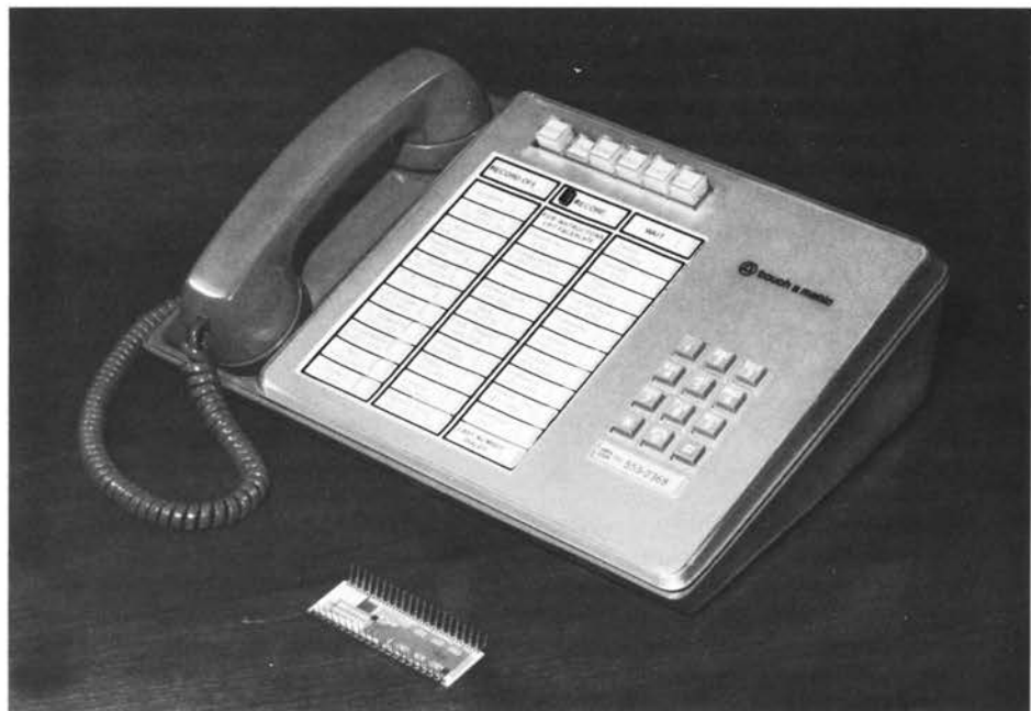
The TOUCH-A-MATIC® set, the first Bell System telephone with a solid-state memory, can dial any of 32 prerecorded numbers at the touch of a button. The memory (foreground) consists of 10 integrated circuits interconnected on a substrate.
